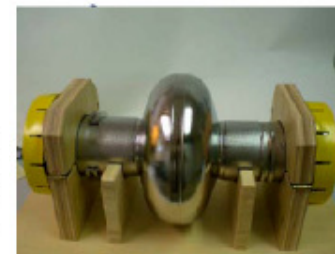
DESY single crystal cavity 1AC8 built from Heraeus disc by rolling at RWTH, deep drawing and EB welding at ACCEL
