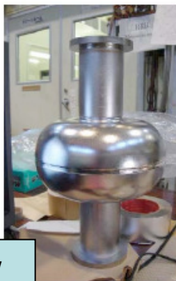
60mm-Aperture Re-Entrant Cavity, 58 MV/m! KEK/Cornell Collaboration
