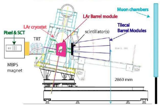
A full slice of the ATLAS experiment has been tested with beams of different particles ( $\pi$ 's,  $\mu$ 's,  $\gamma$ , electrons and protons), at different energies (1-350 GeV) and polarities.
