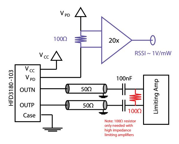
Optional RSSI implementation is shown in blue – implemented in HFD3180-103 only Optional  $100\Omega$  differential termination for high impedance limiting amplifiers is shown in red.
