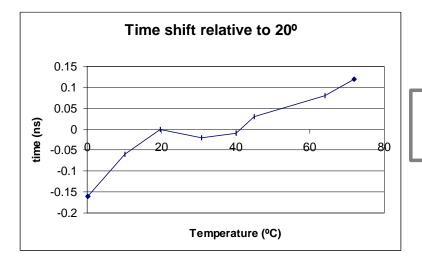
~30% of the time shift is due to DS90LV048A differential line receivers
