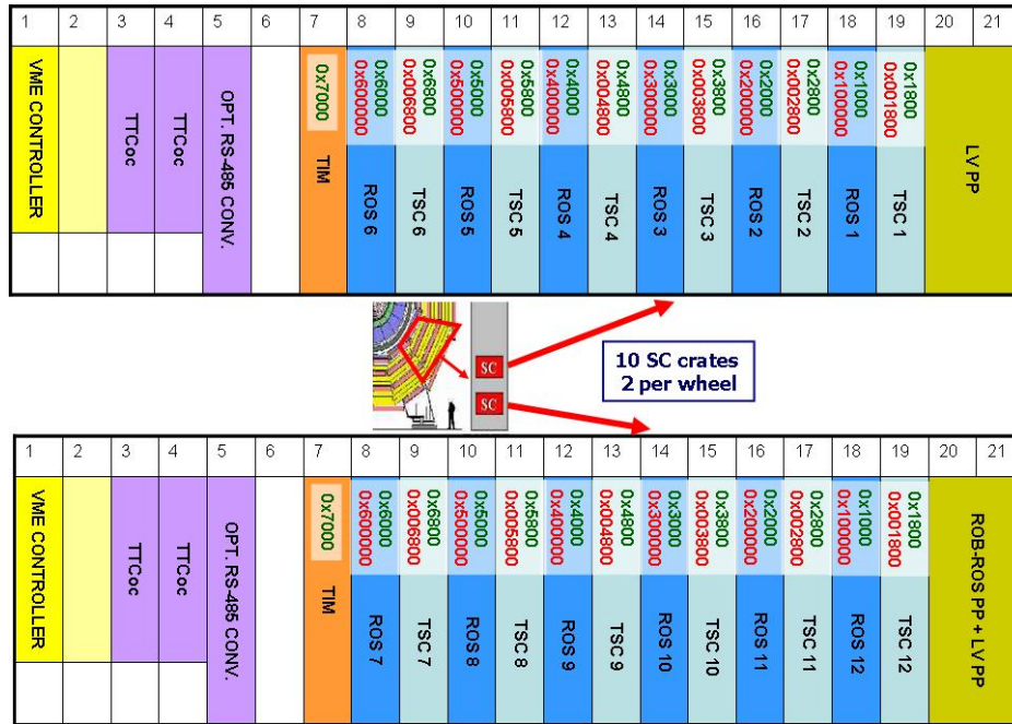
Figure 3: Diagram of the Sector Collector crate with its boards VME base address.
