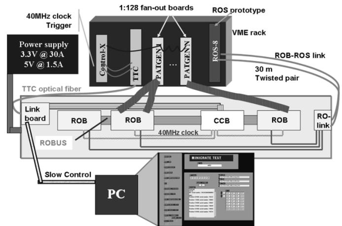
Fig. 5. Diagram of the read-out MC test system.
