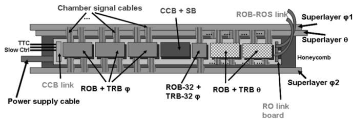
Fig. 3. A schematic drawing of an MB1 MC attached to a chamber is presented in this figure. The three superlayers of the chamber, as well as the honeycomb structure are shown. The different boards and the main connections are indicated.
