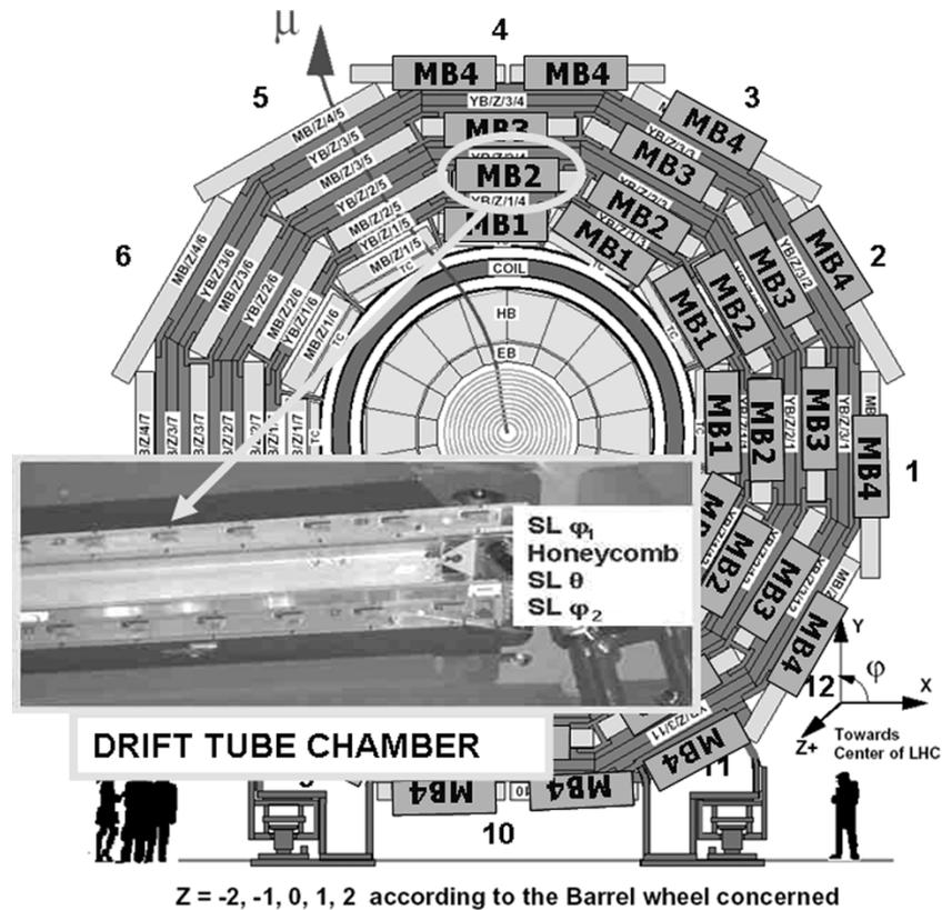
Fig. 1. Transversal view of one of the wheels in the CMS detector barrel region. A picture of a drift tube chamber inserted on the wheel is shown.
