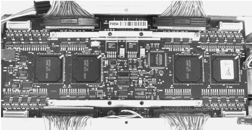
Fig. 2. Picture of a 128-channels ROB assembled on a MC. The two horizontal aluminum pieces that screw the ROB to the MC behave as thermal reliefs for heat dissipation.
