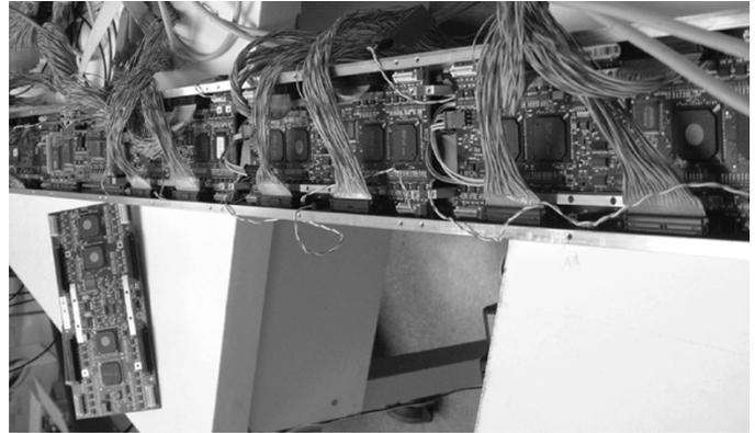
Fig. 4. View of a read-out MC under test.
