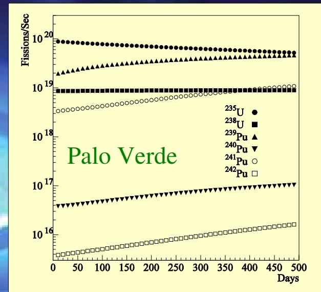
• High flux:  $1\text{GW}_{\text{th}} \sim 2 \times 10^{20} \bar{\nu}_e / \text{s}$
