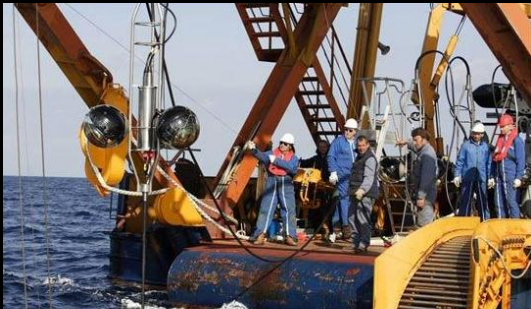
SEEING THE LIGHT Antares's light sensors are designed to detect charged particles created when neutrinos decay, but can be adapted to pick up light from bioluminescent organisms such as jellyfish and bacteria
