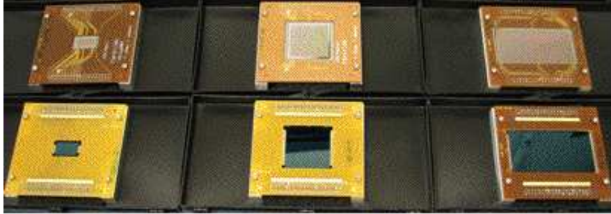
Figure 8: Six different pictureframe package types.
