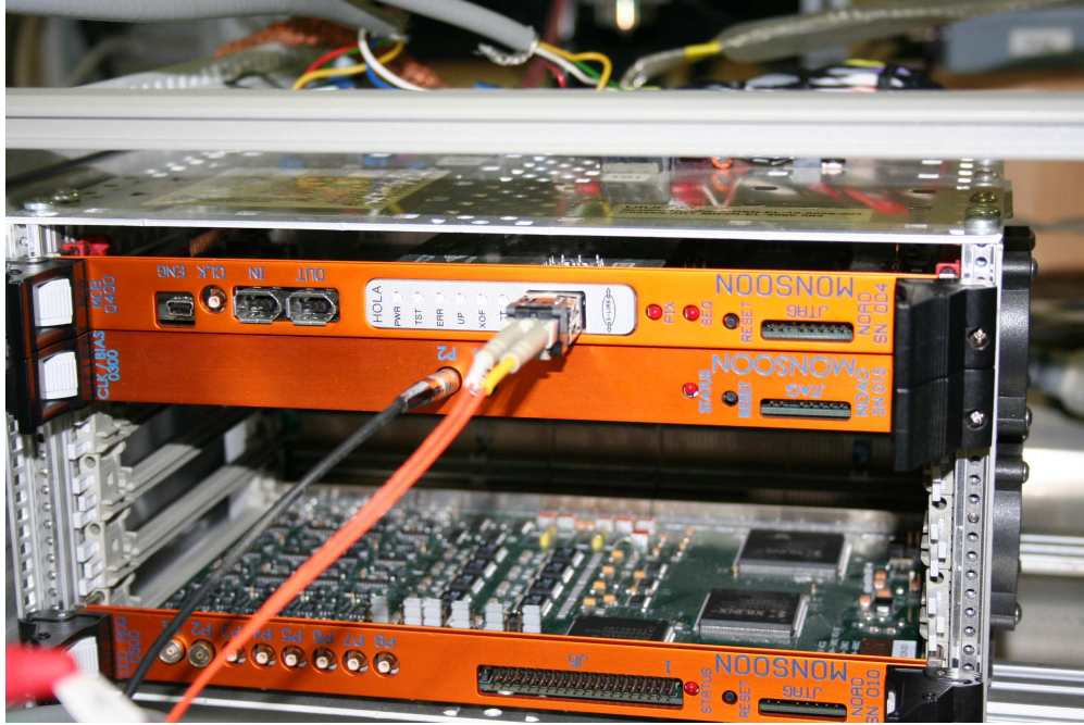
Figure 22: Monsoon Readout System with S-Link and 8-Channel ACQ Board.
