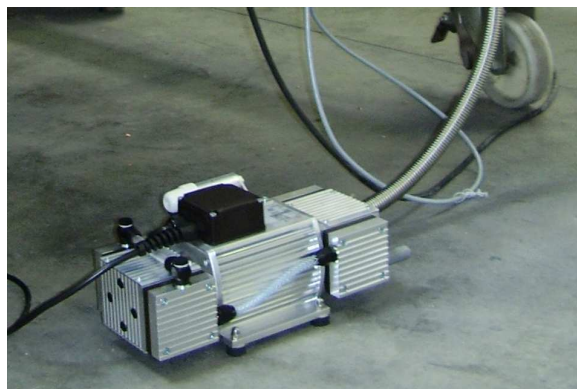
Figure 19: Diaphragm pump and hose that connects with the turbo pump.
